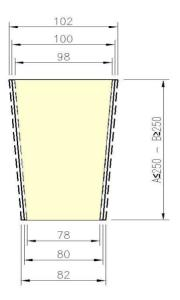
Example for Arches less than 12 Kg - Tolerances for tapers with:  $\pm$  1 mm and  $\pm$  2 mm
